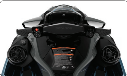
10.25" Touch Display with waterproof audio system Levels up entertainment and connectivity on the water. It includes a factory-installed, truly waterproof Bluetooth® audio system of two 50-watt speakers, a 10.25" touch display and a USB port.
