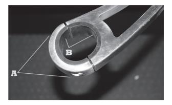
3. Place mounting collar on tower and replace hex head cap screws (A). Snug the collar for now so you can rotate it to the desired location, but tighten screws before using. It is important to tighten the screws evenly or collar may bend, causing thread damage. A small gap between mounting collar halves will remain when tightened properly.
