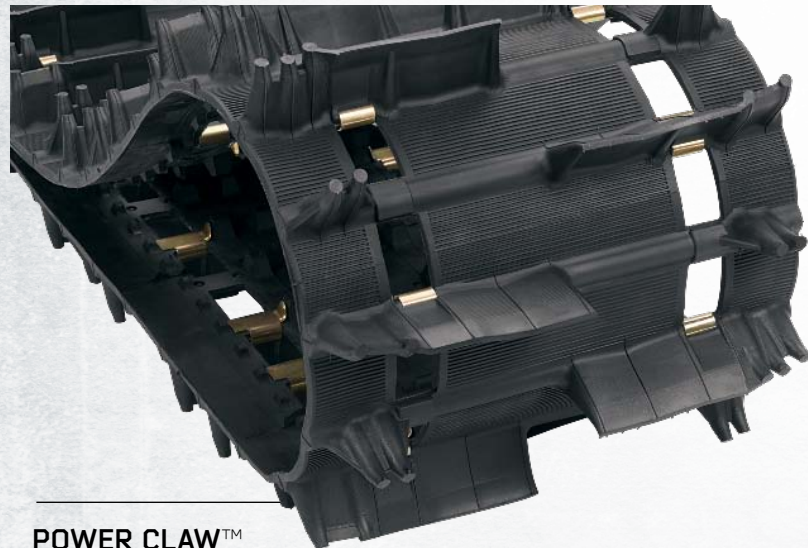
POWER CLAW™ -Phenomenal, lightweight deep powder performance from a 3.0-in. pitch -Excellent sidehill grip from 2.25-in. stagger-set, curved forward paddle towers -Longer useful track life, as it won't fold over and take a set -Snow-cupping outside paddle angles -Free-wheeling track from single-ply technology requires much less horsepower
